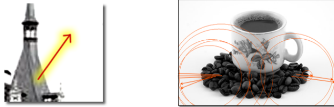
FIGURE 2.7: Example of a detected keypoint. It is represented using a vector that shows the direction on which the difference of intensities is pointing to and how strong that change is (norm of the vector)
