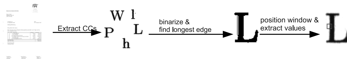
Figure 2.2: General overview of the feature extraction process. First the connected components (CCs) are extracted, then the binarized image is searched for the longest vertical edge. Finally the grey level values are extracted from the middle of the longest edge.
