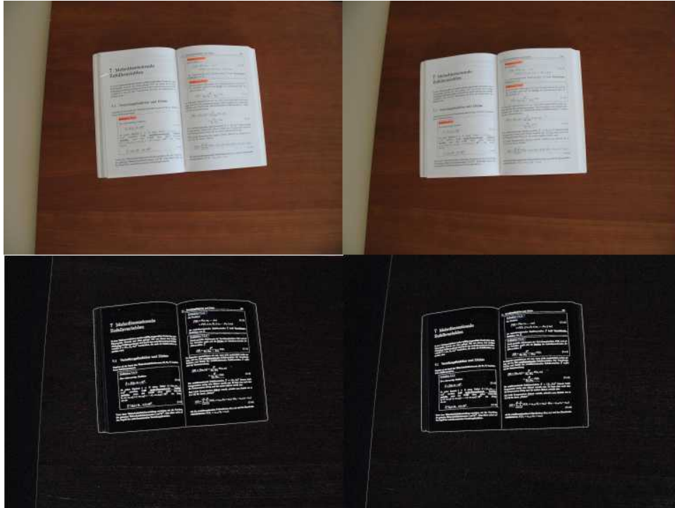
Figure 10: This figure shows an image pair taken by our stereo system and images of edges detected by RAST.
