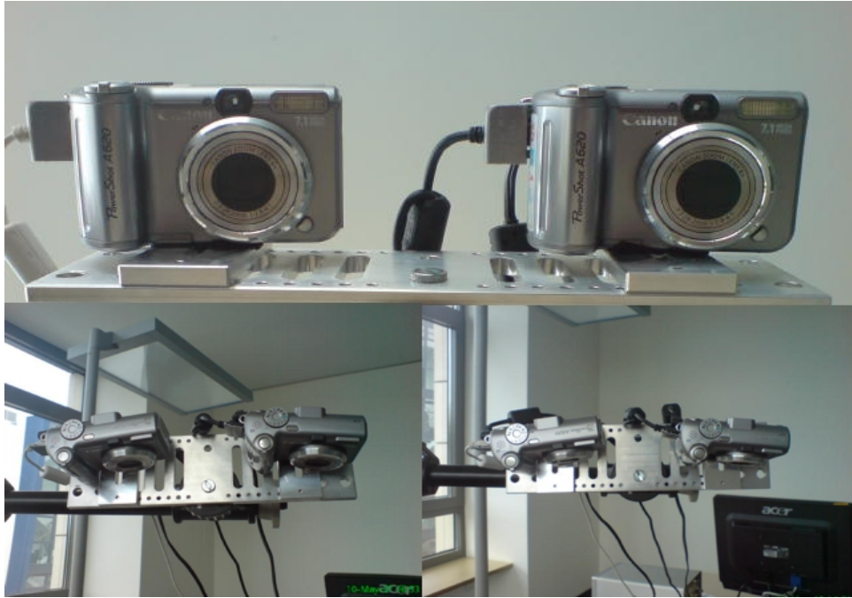
Figure 5: Our stereo system for stereo view. Both cameras covers the same view thus enabling us to get a good 3D model
