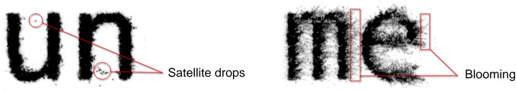
Figure 3.5: Typical inkjet printing defects: (l) satellite drops induced by unclean ink ejection and (r) ink blooming/bleeding resulting from inappropriate ink absorption of the paper.
