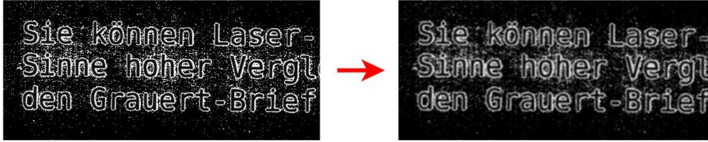
Figure 6.2: Exemplary (l) photocopied document image extract and (r) the obtained denoised result filtered with a  $5 \times 5$  Gaussian filter mask with  $\sigma = 2$ .
