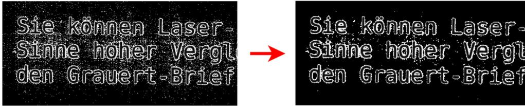
Figure 6.3: Exemplary (l) photocopied document image extract and (r) the obtained denoised result filtered with a  $3 \times 3$  median filter mask.
