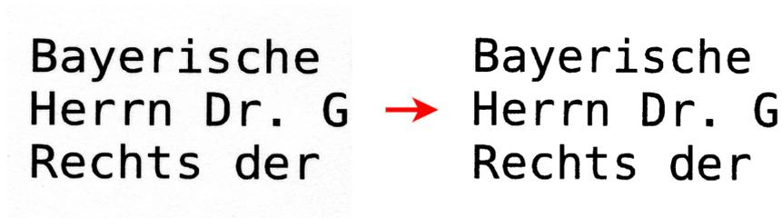
Figure 5.2: Exemplary extract of a binarized document image obtained utilizing Otsu’s [62] binarization approach: (l) original document image (r) binarized result.
