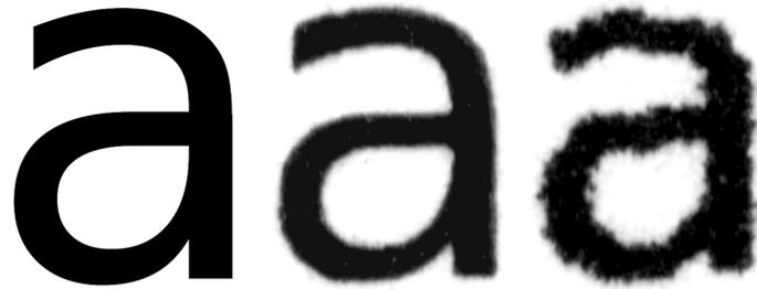
Figure 1.4: High resolution printing technique comparison illustrated by the printed character 'a' scanned at 4800dpi: (l) template character, (m) laser and (r) inkjet printed result.
